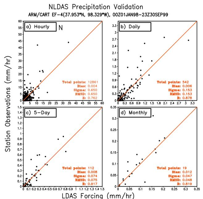
**Figure 4.** Comparison of NLDAS forcing with local forcing for precipitation for station EF-4 of ARM/CART at Plevna, Kansas, representative of other stations. For the hourly panel, each point is for one hour during the period 0000 UT, 1 January 1998 through 2300 UT, 30 September 1999. For the other panels, the averaging period is indicated.
