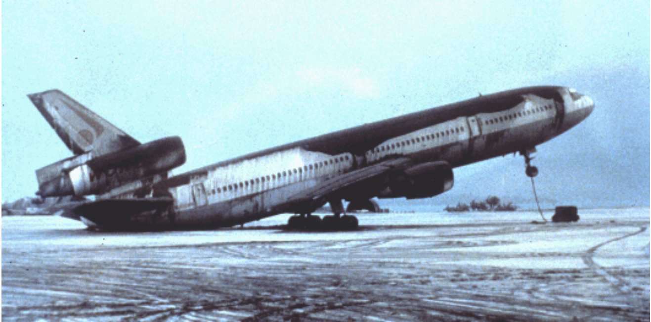
Figure 2. A World Airways DC-10 at Cubi Point Naval Air Station, 40 km from Mt. Pinatubo, tipped backwards from the volcanic ash on the stabilizer. What appears to be snow is actually volcanic ash on the ground. These large particles, while producing devastating local effects and short-term weather effects, fall out of the atmosphere too quickly to affect climate. [U.S. Navy photograph by R. L. Rieger]
